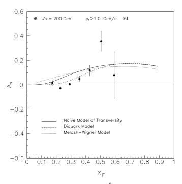
Fig. 4. Single spin asymmetry for  $\pi^0$  [20] in the framework of the two component model with three different transversity parametrizations [15–18, 31–40]. The center of mass energy of the reaction is  $\sqrt{s} = 200 \text{ GeV}$
